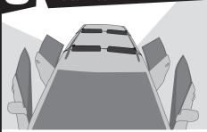
Open all doors on both sides of the vehicle and lay both roof rack pads flat on the roof. They should be parallel to one another, at least 2 ft apart.
