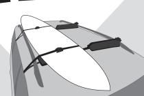
Place your cargo on the pads top side down. Position the buckle center of the board, secure the strap over the board and loop into the buckle from the bottom slot. Pull tight. Always secure and hide the excess straps inside the car.
